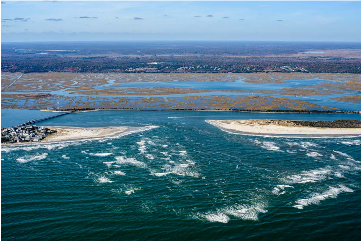
Figure 16. This October 30, 2022 photograph of Corson's Inlet shows the constriction of the main tidal channel by the surrounding ebb-tidal shoal system. Notice the absence of a clear navigable pathway out between Ocean City and northern Ludlam Island to the oceanfront. (Photo by Ted Kingston)
