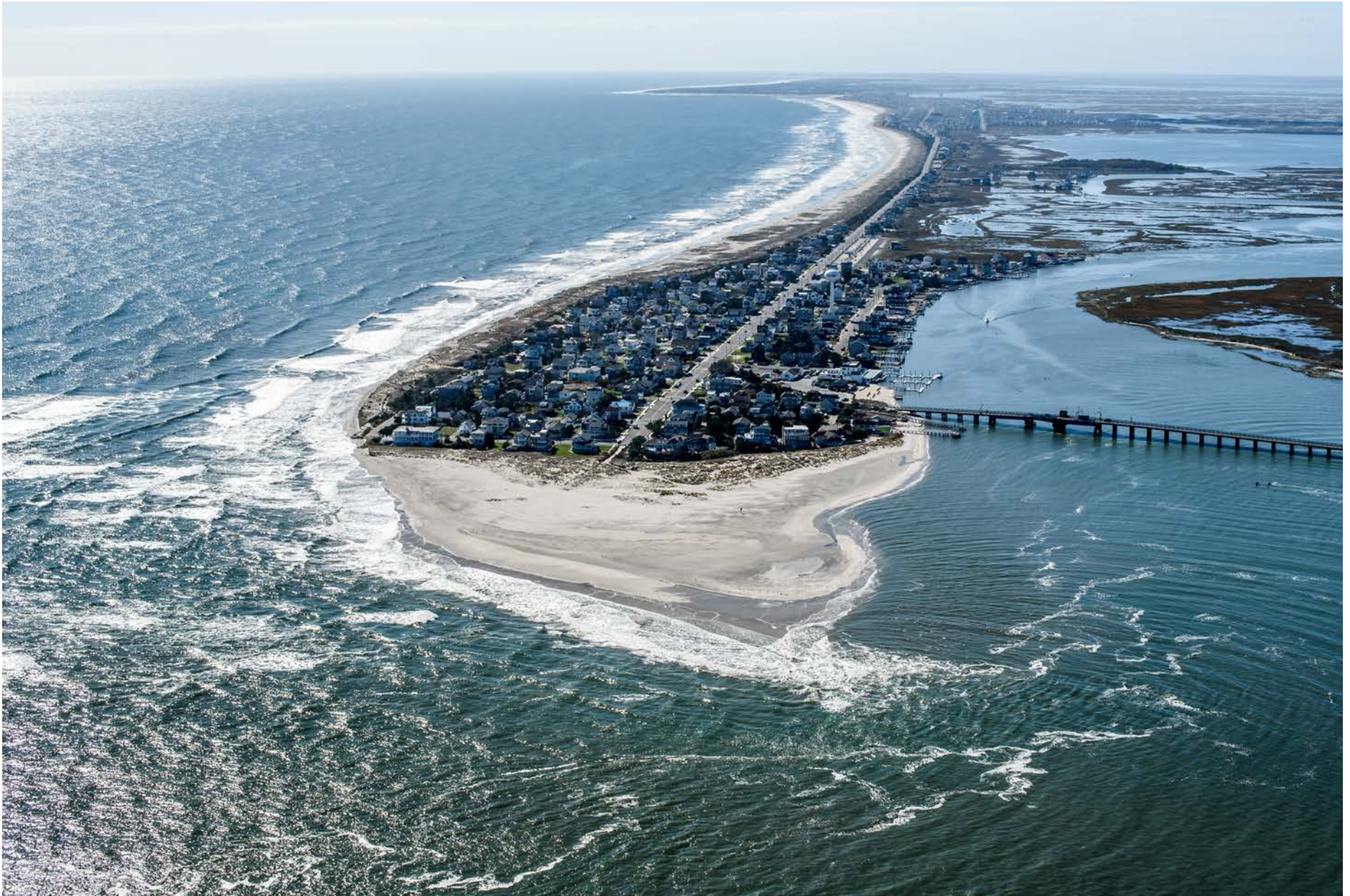
Figure 4. Aerial view of Seaview Avenue profile beach October 30, 2022, looking to the south over Corson's Inlet. The incoming breaking waves and their angle to the shoreline beach combined with the flood-tidal currents moving into Corson's Inlet, generate rapid sand transfer away from this critical region. While shallow wave-like bars still lie just offshore, the beach berm has been cut into a vertical scarp right at the end of Seaview Avenue. That scarp continues into the NJ State Park land to the northwest. Significant volumes of new sand moving north toward the inlet from the southern bar system is required if the erosion is not to move into the 2019-2020 USACE rebuilt dunes this winter.
