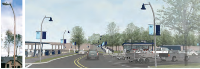
STREET AND AREA LIGHT: TIMBERWOOD PRODUCTS CURVED WOOD POLE WITH STERNBERG OMEGA LUMINAIRE AND CUSTOM BANNERS.
