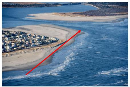
Figure 5. View of Corson's Inlet on December 11, 2018 showing the extent of dune erosion along the same alignment which appeared in September 2017. The impact on the northeast corner municipal dune system is evident. This time there is no subsidary tidal channel along the beach, but also the offshore bar system lies well seaward as seen in the breaking wave pattern.
